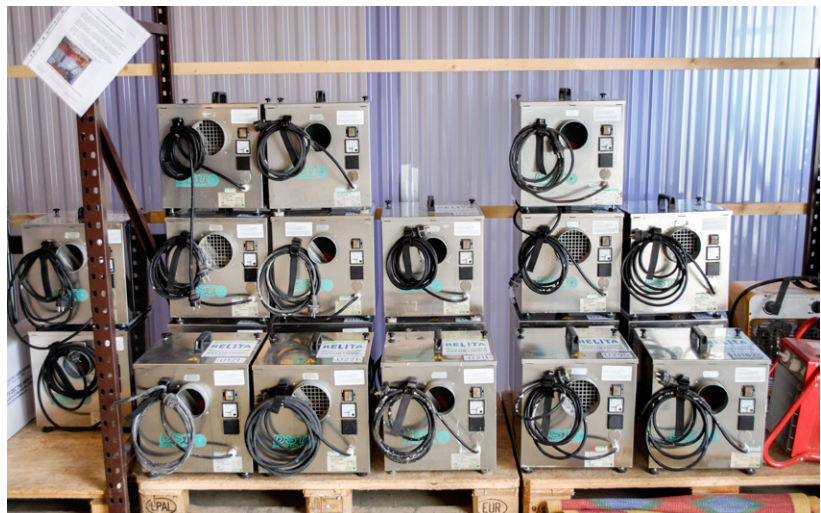
Seibu Giken DST dehumidifier DR-30 ready for the clean-up job with Relita.
